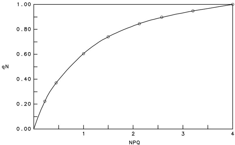
Fig. 18: Relationship between the coefficients of nonphotochemical quenching, qN and NPQ
