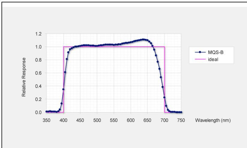
**Fig. 4: Spectral response of MQS-B sensor**
