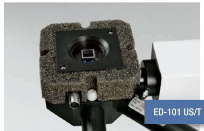
Temperature Control Block Mounted on Optical Unit for Suspension
