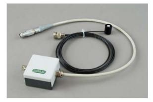
Fig. 6: Mini Quantum Sensor US-MQS/WB
