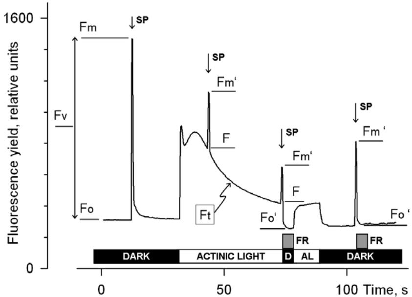
Figure 3.1: Measurements for Saturating Pulse Analysis. AL, actinic light; D, dark; SP, saturating pulse; FR, far-red illumination.
