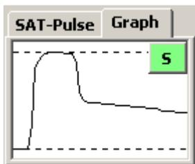
12 different intensity levels are available. Pulse width can be adjusted from 0.2 to 2 seconds. The <SAT-Pulse> defaults (intensity level 10 and 0.8 seconds pulse width) work well with most samples. The fluorescence transient reaches a plateau and does not drop at the end of the saturating pulse interval (Graph interval set value 2.5 s).
