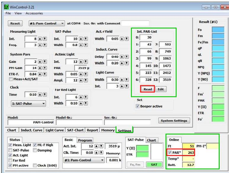
Figure 2.6: Calibration of the Internal PAR-list
