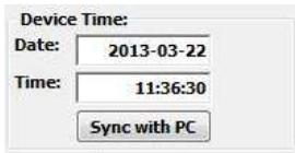
Device Time: shows Date and Time stored in the PAM-CONTROL Unit. The Sync with PC button adjusts Date and Time according to the connected PC.
