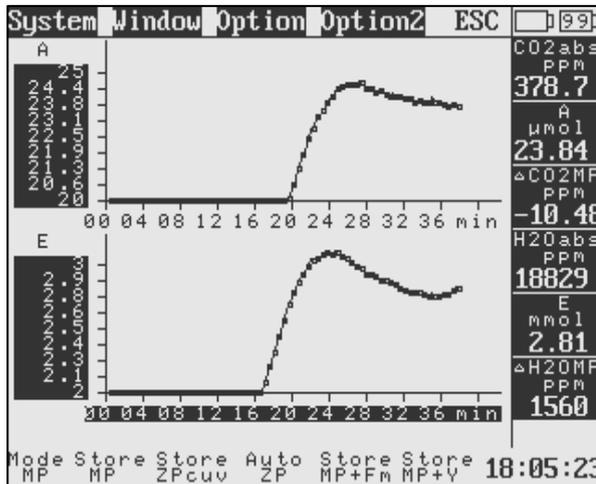
Fig. 8: *Chart window*, A (CO<sub>2</sub>-Assimilation) and E (H<sub>2</sub>O-Evaporation) being displayed.
