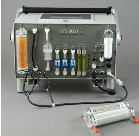
Fig. 21: Set-up for H<sub>2</sub>O zero calibration with air-cycling .
