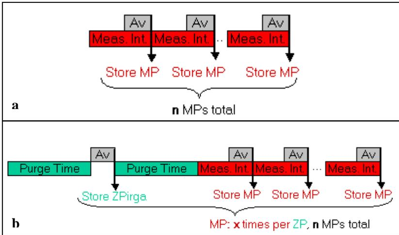
Fig. 5: Illustration of measuring sequences, **a**: sequence 1, **b**: sequence 3.
