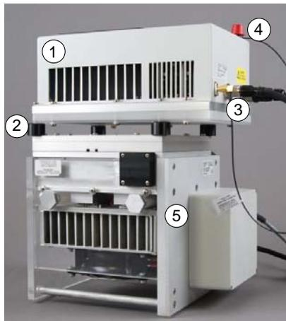
Fig. 1: Mounting LED-Panel RGBW-L084 with an attached Micro Quantum Sensor (MQS/B - optional) on top of Gas-Exchange Chamber 3010-GWK1
