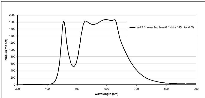
Fig. 10: Spectral distribution of the LED colors mix: red 03, green 14, blue 6 and white 145 at total brightness of 50%
