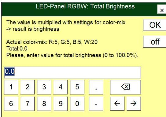
Fig. 5: Dialog window LED-Panel RGBW: Total Brightness
