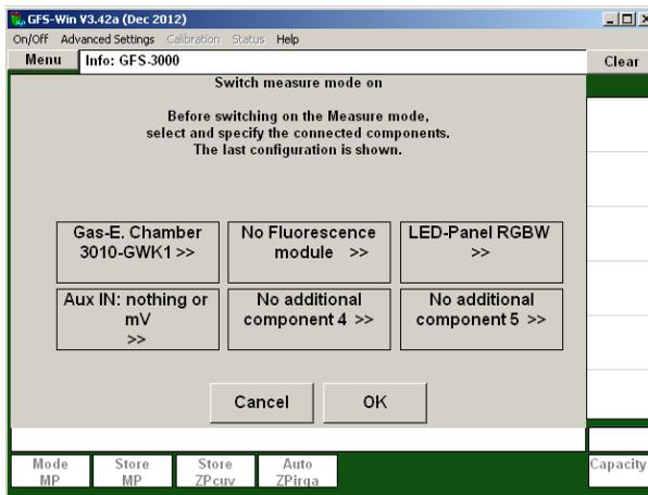
Fig. 2: Choosing Gas-E. Chamber 3010-GWK1 and LED-Panel RGBW in GFS-Win and on the Panel PC
