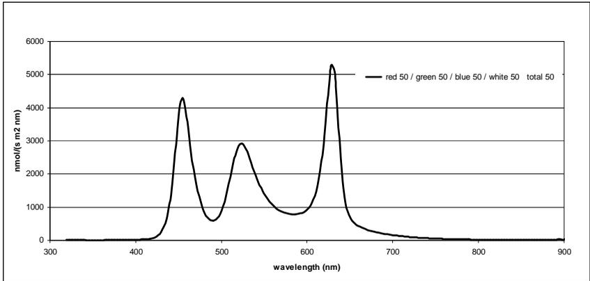
Fig. 9: Spectral distribution of the LED colors: red, green, blue and white measured together at intensity step 50, total 50%
