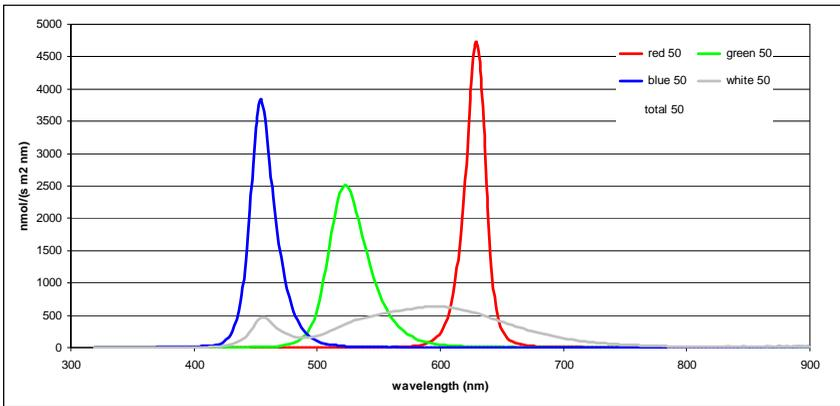
Fig. 8: Spectral distribution of the LED colors: red, green, blue and white each measured at intensity step 50, total 50%
