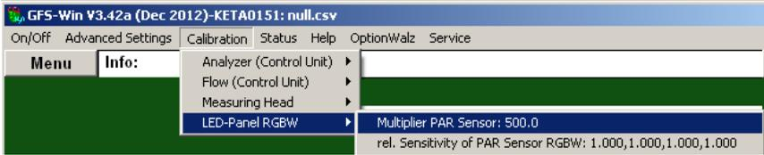
Fig. 7: Multiplier for external PAR-sensor of LED-panel.
