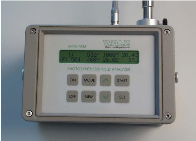
Fig. 1: Photosynthesis Yield Analyzer MINI-PAM
