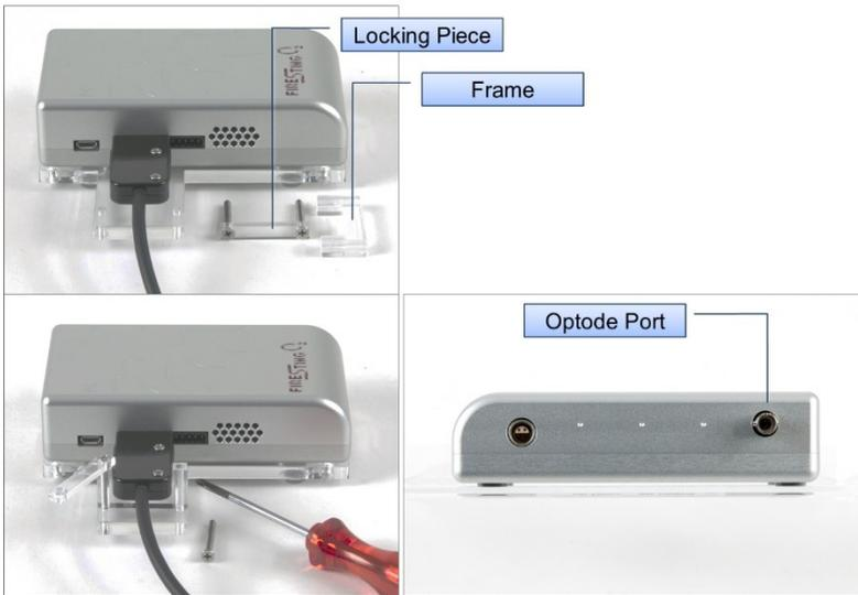
**Fig. 8: Mounting the Interface Plug**
