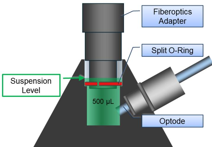
Fig. 12: Suspension Level
