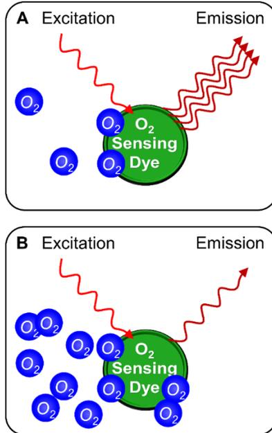
**Fig. 1: Principle of O<sub>2</sub> Detection**
