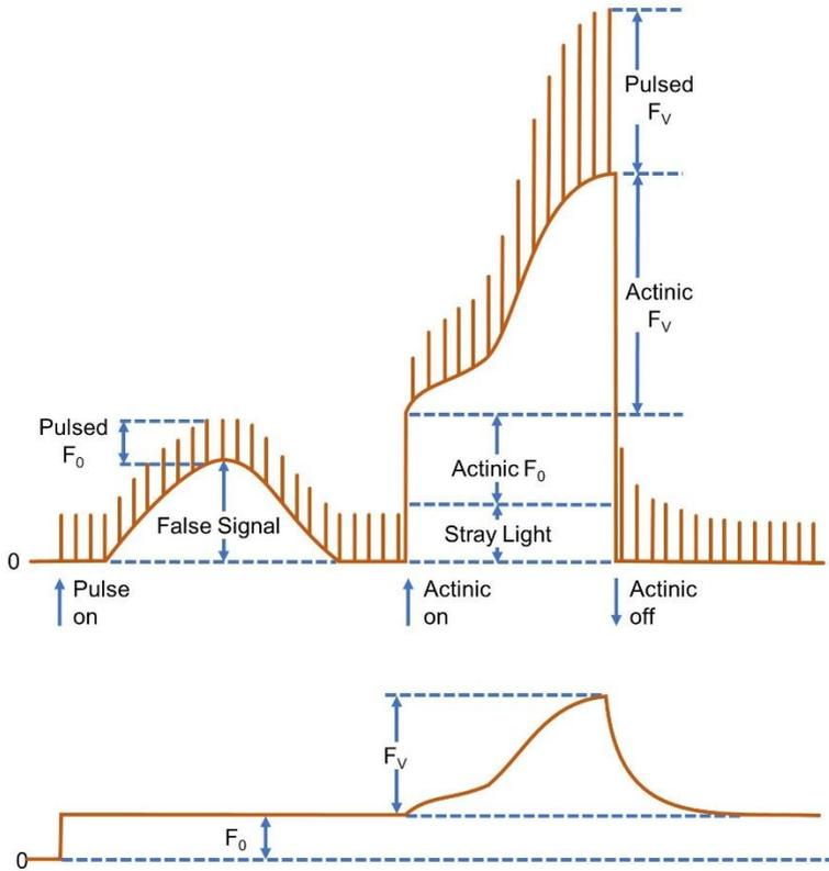
**Fig. 2-8: Illustration of the PAM measurement principle.**
