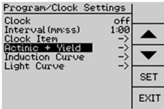
The menu “Program/Clock Settings” provides all options to configure automated experimental routines like Actinic + Yield, Induction Curve and Light Curve experiments as well as repetitive triggering of single measurements and
