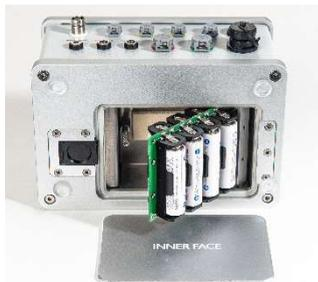
To open the battery compartment, shift the closing mechanism to the side.
