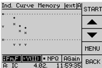
MEM of the Induction Curve window opens the “Ind. Curve Memory” window. In this window, the navigation keys permit scrolling through stored induction curves. The experiments are annotated in the information line by date and time of the measurements. There are two options to leave the Ind. Curve Memory window, either by pressing “START” to measure a new induction curve or by using the “BACK” key to return to the last measured induction curve data.
