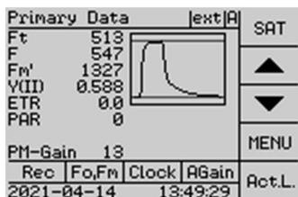
This window shows the values of the current Ft signal, a depiction of the fluorescence trace of the last saturation pulse, resulting data (F, Fm', Y(II), ETR) and instrumental parameters as
