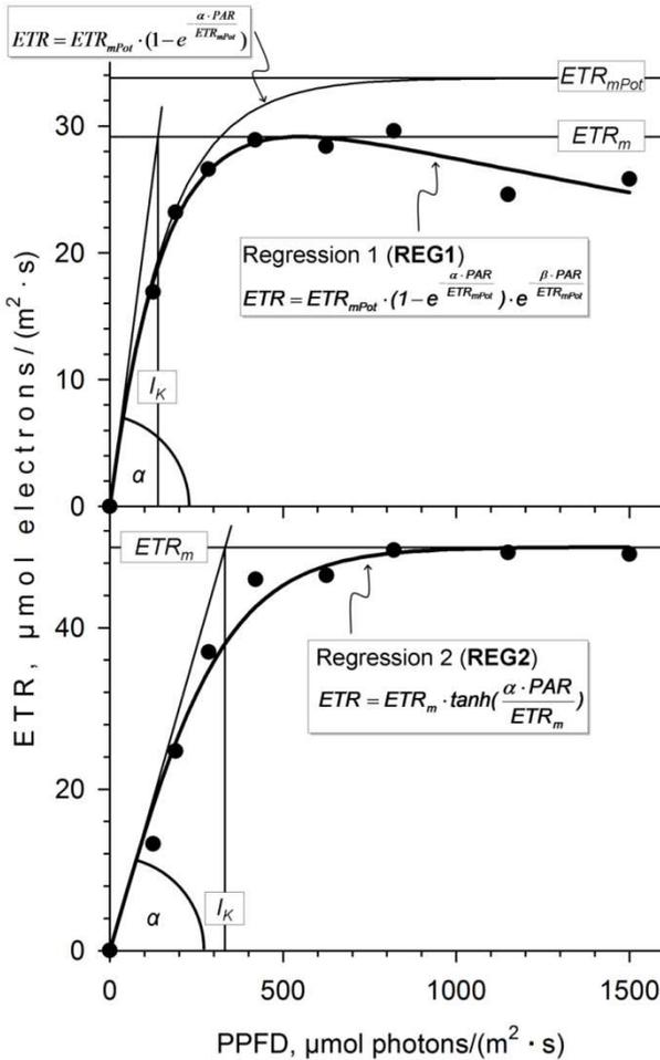
Fig. 14: Model Functions of Rapid Light Curves
