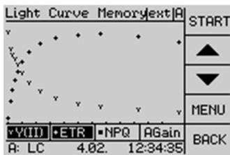
In the light curve window MEM opens the memory of light curve experiments. The navigation keys permit scrolling through stored light curves. The experiments are annotated in the information line by date and time of the measurements. There are two options to leave the memory window, either by pressing “START” to measure a new light curve or by using the “BACK” key to return to the last measured light curve data.
