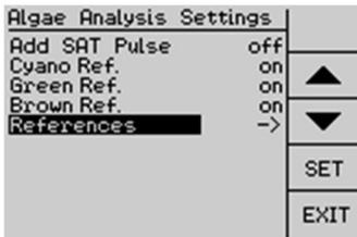
This menu refers to the differential algae content determination. The chlorophyll content measurement can be combined with a saturation pulse analysis. When the menu item “Add SAT Pulse” is marked with yes the WATER-PAM-II will automatically append a saturation pulse for determination of the photosynthetic performance of the sample.
