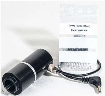
The stirrer is powered and controlled by WATER-PAM-II. Please connect the stirrer plug to the stirrer port on the rear side of WATER-PAM-II. The disposable paddle can be removed by gentle pulling. The other way around, a replacement paddle can be mounted by pushing the cylindrical end all the way into holder on the upper inside of the stirring device.
