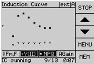
Settings of an induction curve experiment as number of saturation pulse analyses, interval between pulses and the option to continue fluorescence monitoring after the induction curve in the dark (recovery curve) can be adjusted in the menu “Induction Curve Settings” which is available in Main Menu (more information in chapter: 5.4.5).
