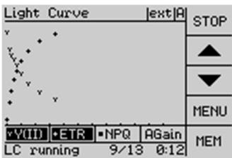
window provides a predesigned procedure to execute a light curve protocol. Relevant parameters (number and duration of light steps, initial PAR, and recovery curve) can be adjusted in the menu “Light Curve Settings” (chapter
