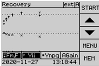
Fluorescence recovery experiments are often appended to induction or light curves. In Water-PAM-II instruments this can be chosen in the menu light-/induction curve settings (chapter 5.4.5 and 5.4.6). In these cases, recovery curves are started automatically and resulting data is displayed in the Recovery window.
