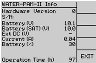
This window provides information about the hardware version and serial number of the instrument in line 1 and 2. Line 3-6 show power related details:
