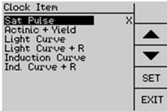
Saturation pulse analyses and the programs Actinic + Yield, Induction Curve and Light Curve can be repetitively performed under clock control. Also, recovery experiments can be performed after induction and light curves (item
