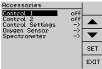
Accessories include settings of components that could be connected to the WATER-PAM-II in addition to the standard components like components controlled by PWM signal (CTRL ports), spectrometer, oxygen sensor etc.
