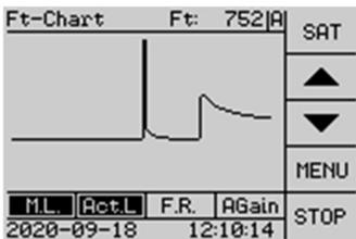
The X axis interval can be adjusted in the main menu “Instrument Set” to 0.2 or 1.0 s/dot Ft chart resolution corresponding to 25 or 125 s/total time axis (chapter 5.6.1). The Ft: value above the graph corresponds to the current Ft value.
