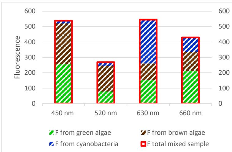
Fig. 8: Example of group specific contribution of F signal to overall F value, fitted with typical reference spectra
