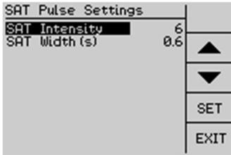
Moving to “SAT Sett.” and SET opens the submenu “SAT Pulse Settings” in which relative intensity (1 to 12) and duration (width, 0.2 to 2.0 s) of saturation pulses can be set.
