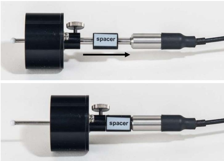
Fig. 10: Mounting of US-SQS/L, 15.3 mm spacer
