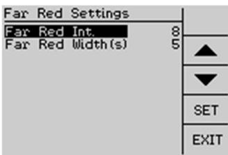
Opens submenu to adjust intensity and duration of far red illumination. These settings are active in  $F_0'$  determinations. The FR light intensity can be adjusted in 12 intensity settings steps. Please marked item Far Red Int. by the up/down arrows
