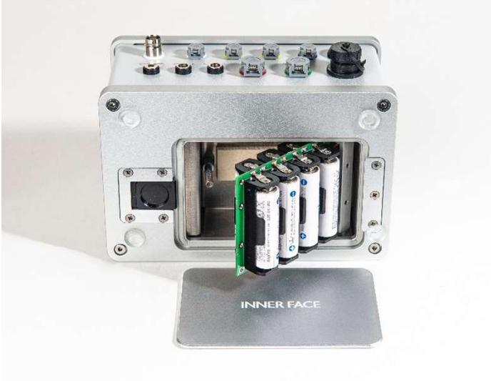
As the optoelectronic unit provides no charging function the system can always be operated, also in presence of non-rechargeable batteries, by mains power via mains power supply MINI-PAM-II/N.
