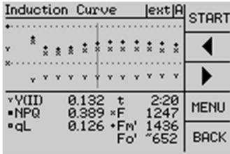
For quantification, all induction curve windows also provide numerical data of fluorescence ratio parameters and fluorescence levels.
