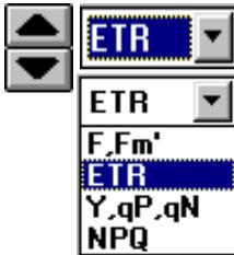
With the help of the **vertical arrow keys** the scaling of the **Y-axis** can be modified within wide ranges. The **selection box** located underneath the arrow keys allows to choose between the scales of different parameters (F and Fm', ETR, Y, qP, and qN, as well as NPQ). Please note that the vertical arrow keys are not functional when the Y, qP, qN scale is selected, as in this case the scale is always ranging from 0 to 1.
