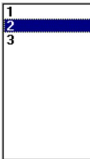
The **Select** box shows a list of the recorded Chart Curves. A particular curve can be selected by mouse click and then will be displayed. With the keys Pos.1 and End one can jump to the first and last curve, respectively.
