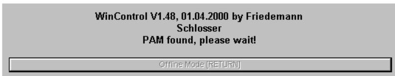
The program automatically compares the time and date set via the instrument software (EPROM) with that of the PC and recognizes that there are differences. As it is important that stored data are characterized by the same time and date in instrument and PC memory, the suggestion to correct the PAM date and time (synchronize with PC) should be answered with Yes.
