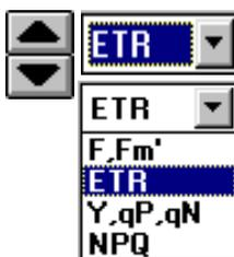
With the help of the **vertical arrow keys** the scaling of the **Y-axis** can be modified within wide ranges. The **selection box** located underneath the arrow keys allows to choose between the scales of different parameters (F and Fm', ETR, Y, qP and qN, as well as NPQ). Please note that the vertical arrow keys are not functional when the Y,qP,qN scale is selected,
