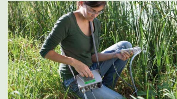
The MINI-PAM-II fluorometer combines the advantages of its predecessor with most recent LED and computer technology. A transfective touchscreen, energy efficient LED sources and easy replaceable off-the-shelf batteries make the MINI-PAM-II the ideal PAM fluorometer for field research. All common fluorescence parameters are automatically calculated.
