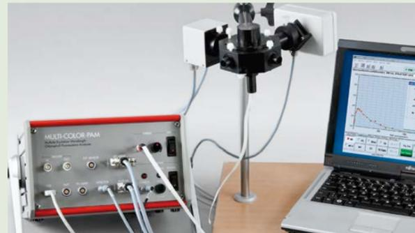
The MULTI-COLOR-PAM provides six colors of pulse-modulated measuring light (365 or 400, 440, 480, 540, 590 and 625 nm) and five colors of actinic light (440, 480, 540, 590, 625) plus white (420-640 nm) and far-red light (730 nm).
