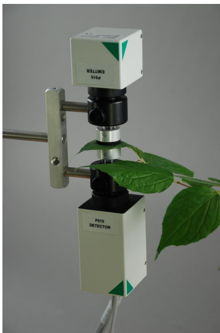
Fig. 1. Emitter unit DUAL-EP515 and detector unit DUAL-DP515
