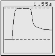
The saturating light pulse serves to fully reduce photosystem II. It is activated with the button *Store MP+Fm* or the button *Store MP+Yield* at the bottom of the screen. After every saturating light pulse, the kinetic of the fluorescence signal is displayed in a small graph.
