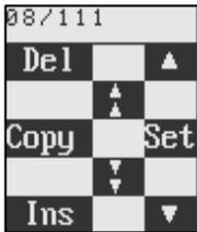
The arrow keys serve to navigate within the program listing. The number in the upper line, here 08/111, indicates which line is selected and the total amount of lines in the user-program. *Del* deletes the selected line, *Copy* copies the selected line. The line copied to the memory is shown in the line above the bottom bar. With *Ins* it can be inserted multiple times. With *Set* the selected line of the program listing can be changed.
