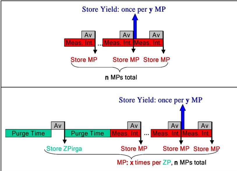
Fig. 7: Illustration of Measuring Sequence, with automatic yield measurements
