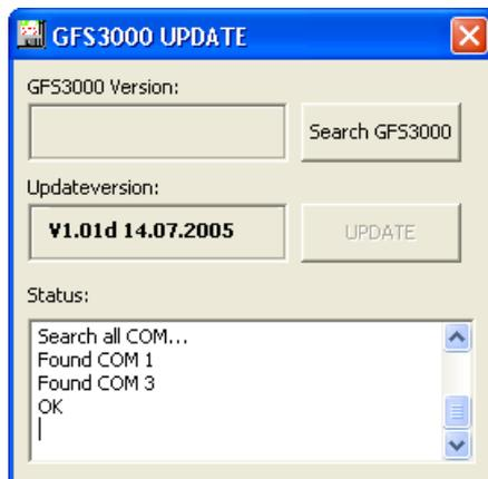
pressing *OK*. Afterwards press *Search GFS-3000* to find the currently installed software version.
