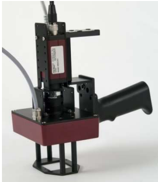
Fig. 27: MINI-Head with CCD camera and grip holder
