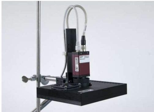
Fig. 6: Measuring Head consisting of LED-Array Illumination Unit and CCD-camera mounted via 15 mm \varnothing metal bar on optional stand (Stand with Base Plate ST 101)
