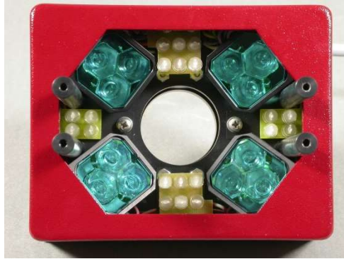
Fig. 18: Top view of MINI-Head IMAG-MIN/B LED-array without aluminum rods holding the sample-platform
