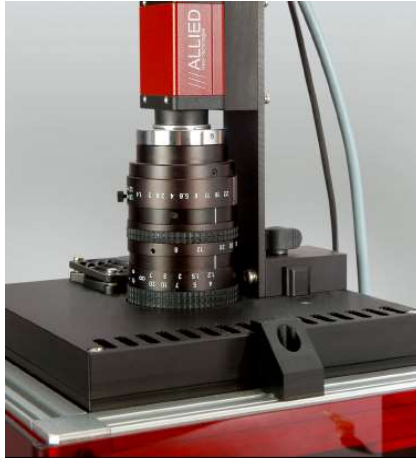
Fig. 11: CCD Camera with Zoom objective
