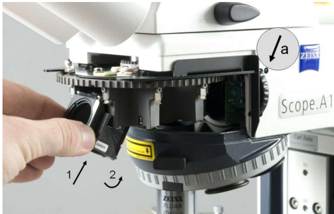
Fig. 51: Mounting the reflector module
