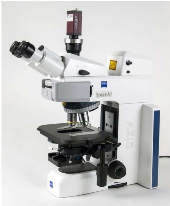
Fig. 46: MICROSCOPY-IMAGING-PAM based on Zeiss ScopeA.1 Epifluorescence Microscope
