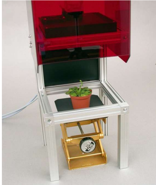
Fig. 15: IMAG MAX/GS, with bottom part being removed, resting on two spacers to give room for potted plant
