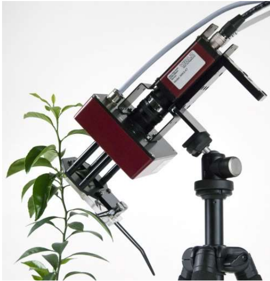
Fig. 29: Mini-Head with Leaf Holder mounted on a tripod
