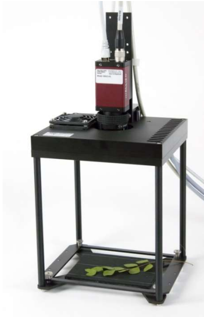
Fig. 16: Leaf Distance Holder IMAG-MAX/B with IMAG-MAX/L and IMAG-K6
