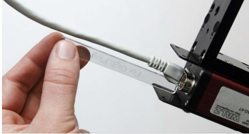
Fig. 21: Perspex device to unplug GigE cable from a mounted camera
