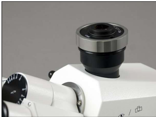
Fig. 44: Zeiss camera adapter mounted on Axio Scope.A1
