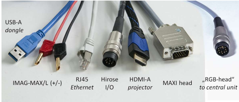
Fig. 38: connectors in cable harness coming from IMAG-3D.
