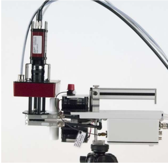
Fig. 34: MINI-Head mounted on Standard Measuring Head of the GFS-3000 Gas Exchange Fluorescence System
