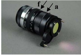
Fig. 22: Standard lens for IMAG-MIN/GFP (focus ring = f , aperture = a ), filter slider in GFP position
