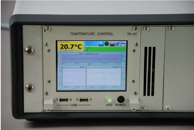
Fig. 12: Panel-PC of Temperature Controller TR-KF-24 with USB connectors and power button
