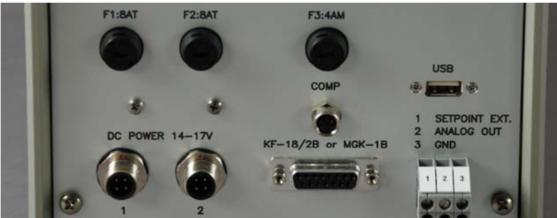
Fig. 15: TR-KF-18: Connectors at the back side
