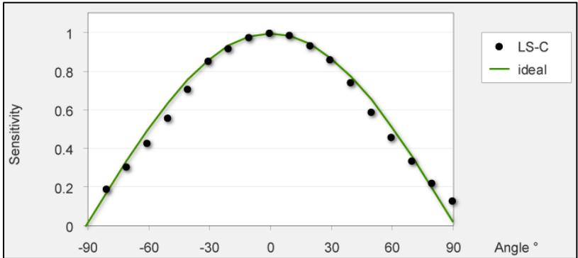
Fig. 3: Typical angular response curve of the mini quantum sensor. The mini quantum sensor uses a plastic diffuser to obtain an angular response error of less than  $\pm 3\%$  (-30...30 ° angle). Dots, actual angular response. Line, ideal cosine response.
