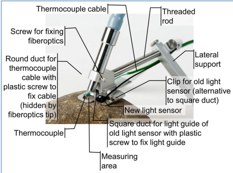
Fig. 5: 2060-A Fiberoptics Holder for Surfaces equipped with light and temperature sensors. The 2060-A clip can also hold first generation “micro” quantum sensors (“old light sensors”).
