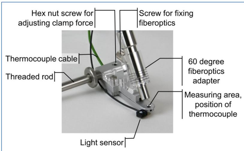
Fig. 4: 2060-B Arabidopsis Leaf Clip equipped with PAR and temperature sensors.
