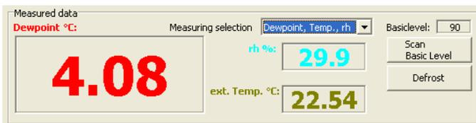
In the case a menu button on the TS-2 control unit is pressed by mistake the communication will be interrupted and values are frozen on the screen. Press “Search all COM” (1.1) and the communication is started from new.
