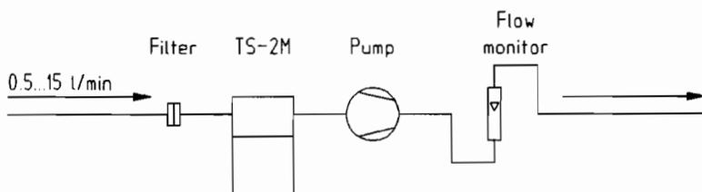
Fig. 4: Integration of the Dewpoint Mirror Measuring Head TS-2M in a pneumatic system with a measuring gas flow of 0.5 - 15 l/min
