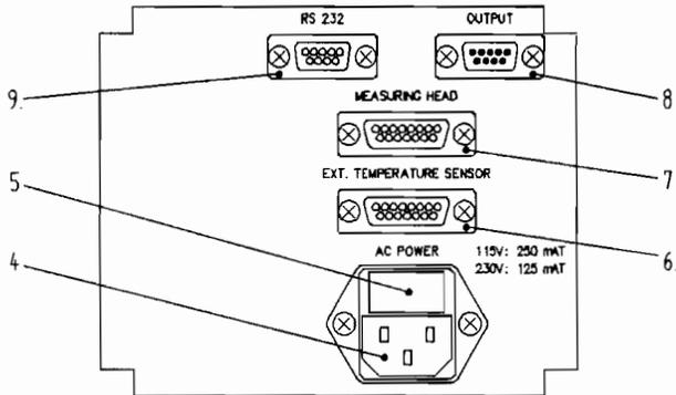
Fig. 3: Rear panel of the Control and Display Unit TS-2
