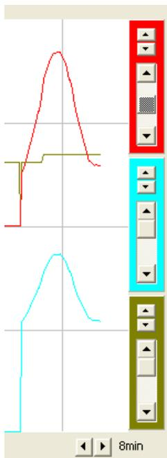
With the Graphics Screen the measured Values (1.2.1 and 1.2.4) can easily be followed. The colors used for the values correspond to the colors used in the “Measured Data” window. With the little Arrow buttons the spreading of the Y-axis can be influenced and with the scroll-bar the position of the curve in the graphic can be determined. The Arrows on the button determine the spreading of the X-axis.
