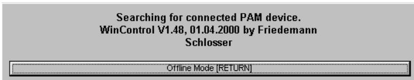
If no PAM fluorometer is connected, the user may select the **Offline Mode** by clicking RETURN. Using this mode it is possible to analyze data which are stored on floppy or PC hard discs. If a PAM is connected via RS 232 interface cable, this will be recognized by the program and it will be automatically switched on:
