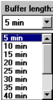
The **Buffer length** corresponds to the time of a full recording which involves 32000 points of fluorescence yield. At the standard buffer length of 5 min this is equivalent to a sampling rate of ca. 100 points/sec.
