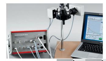
The MULTI-COLOR-PAM provides six colors of pulse modulated measuring light (365 or 400, 440, 480, 540, 590 and 625 nm) and five colors of actinic light (440, 480, 540, 590 625) plus white (420-640 nm) and far-red light (730 nm).
