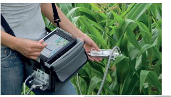
Powerful LEDs providing single turnover flashes for one complete PS II excitation and multipleturnover pulses for O-I<sub>1</sub>-I<sub>2</sub>-P determinations and the standard saturation pulse method.
