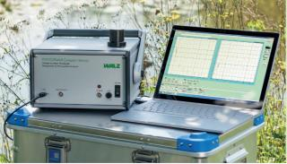
Both PHYTO-PAM-II versions provide five measuring light wavelengths, six actinic light colors, the full range of saturation pulse analysis, assessment of chlorophyll a content, fast kinetics. determination of the functional antenna size of PS II, automated recording, and script file operation.
