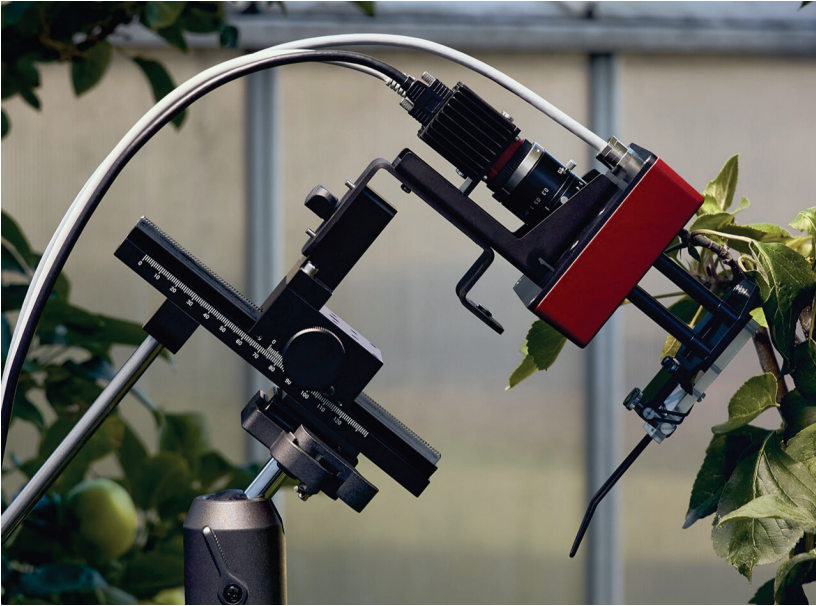
Fig. 33: Mini-Head with Leaf Holder IMAG-MIN/BK and IMAG-MIN/ST mounted on a tripod
