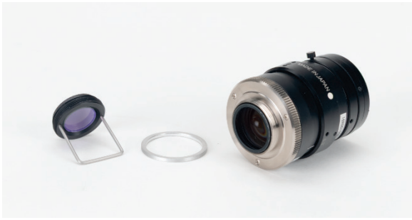
Fig. 12 Kowa prime lens with 16 mm focal length, short pass filter and mounting device (left), distance ring (middle) used with IMAG-K9 CMOS camera on MAXI heads. The distance ring must be placed between lens and camera to enable correct focusing at short distances
