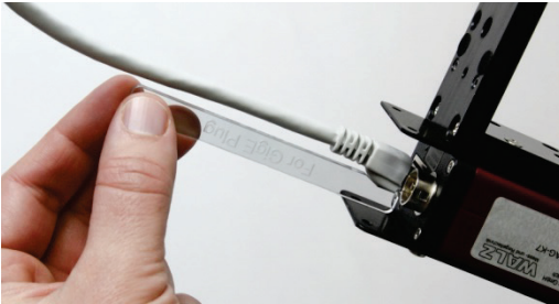
Fig. 27: Perspex device to unplug GigE cable from a mounted camera
