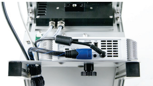
Fig. 48: Rear view of the projector with correct connections for power and HDMI (cable for filter slider actuator is not visible here)
