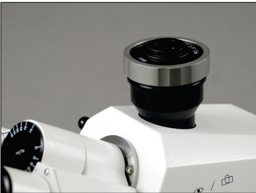
Fig. 53: Zeiss camera adapter mounted on Axio Scope.A1
