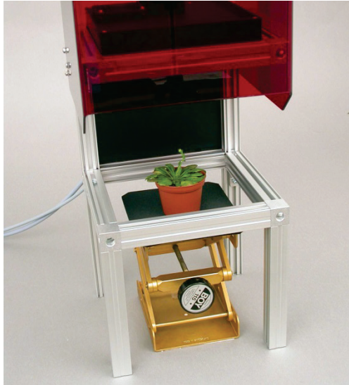
Fig. 21: The mounting stand (IMAG-MAX/GS) is configured for potted plants. The base plate has been removed, and the mounting stand has been jacked up using the additional legs provided with the IMAG-MAX/GS article.
