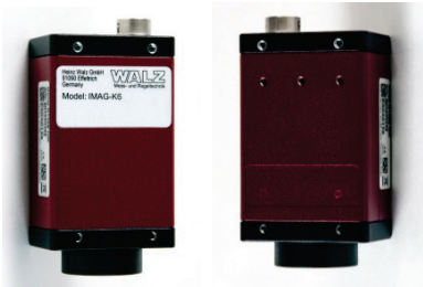
Fig. 25: Camera side with 4 screw holes and label (left) - facing the labelled LED-Array side, camera side with 7 screw holes (right) facing the LED-Array backside and the metal angle bar (Fig. 26 A)
