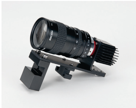
Fig. 14 IMAG-K9 camera with Ricoh zoom lens mounted. Due to their different lengths, the lenses are attached to different positions on the mounting set. The plastic block on the rear is used to hold the cable. It moves to the vacant position during conversion. To use the zoom lens with a MAXI imaging system, the LED array adapter ring must be removed before installation ( Fig. 16).
