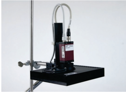
Fig. 8: Measuring Head consisting of LED-array illumination unit and CCD-camera mounted via 15 mm \varnothing metal rod on optional stand (stand with base plate ST 101)
