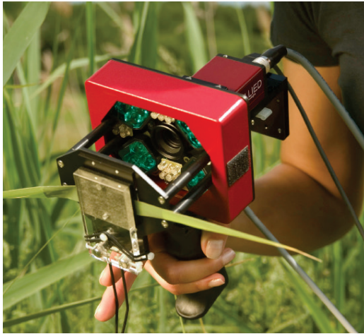
Fig. 32: Mini-Head with grip holder IMAG-MIN/BK used in field
