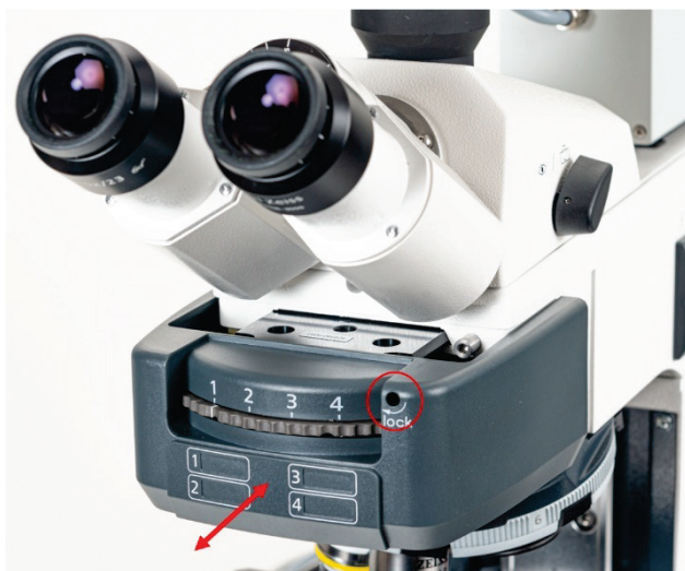
Fig. 61 disassembly of the filter turret of Axioscope 5
