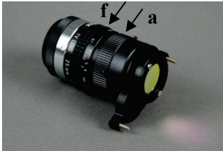
Fig. 38: Standard lens for IMAG-MIN/GFP (focus ring = f, aperture = a), filter slider in GFP position
