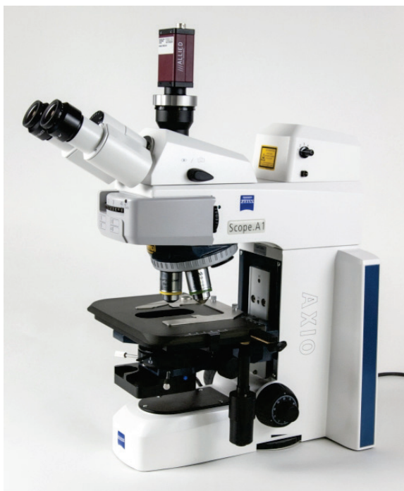
Fig. 55: MICROSCOPY-IMAGING-PAM based on Zeiss ScopeA.1 Epifluorescence Microscope
