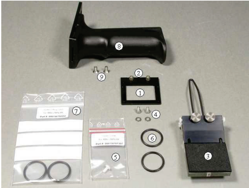
Fig. 34: Components of the Leaf Holder
