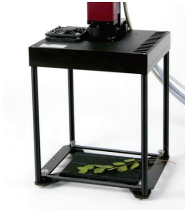
Fig. 22: Leaf Distance Holder IMAG-MAX/B with IMAG-MAX/L and IMAG-K6
