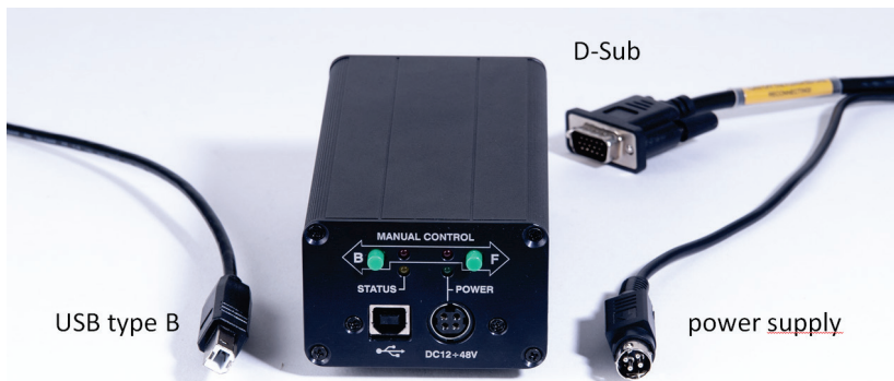
Fig. 51 interface for turntable control
