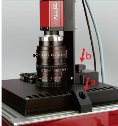
Fig. 17 when setting up the MAXI imaging version it is recommended to mount the LED array on top of IMAG-MAX/GS with the clamps provided (a) and for continuity of measuring configuration also use the wing nut screw to fix the camera
