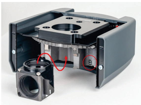
Fig. 62 Mount the push-and-click (P&C) reflector modules delivered with an IMAG-AXIOSCOPE-5 or accessory set IMAG-AX-SCOPE-5
