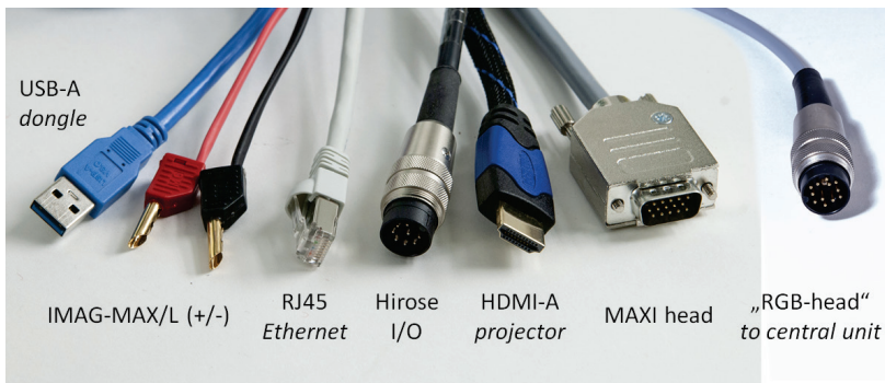
Fig. 47: connectors in cable harness coming from IMAG-3D.
