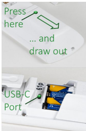
Fig. 12: Access to USB-C Port
