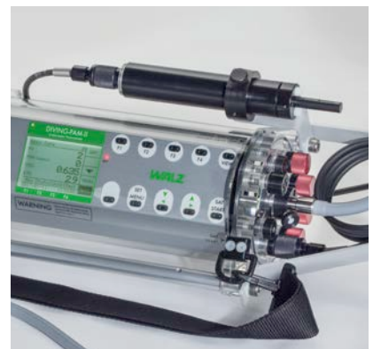
During transport or when surfaces are inspected, the Miniature Spectrometer MINI-SPEC can be conveniently attached to a dedicated holder of the DIVING-PAM-II. The software provides the opportunity to record a light spectrum with each saturation pulse analysis.
