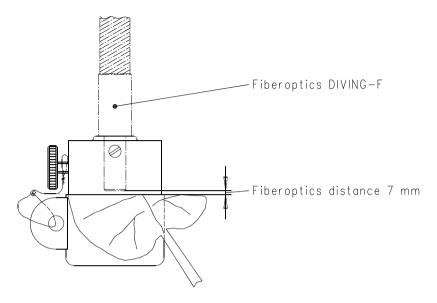
Fig. 6: Magnet Sample Holder DIVING-MLC
