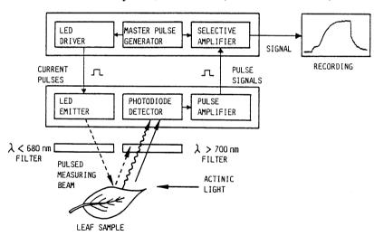
Fig. 16: Schematic view of the PAM measuring principle
