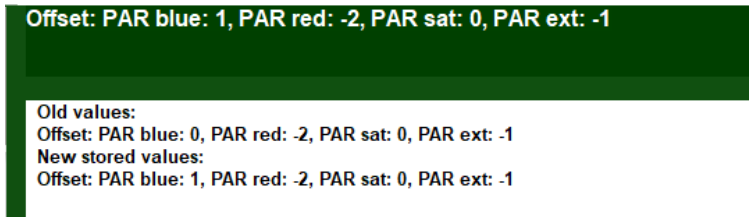
Fig. 16: Result of zero-offset determination for all PAR-sensors of the PAM-fluorometer
