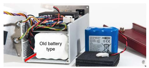
Remove rear panel and put aside. Pull out old battery.
