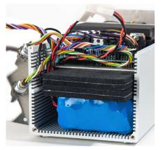
Insert new battery as shown. Foam plates, supplied with the battery, must be inserted <u>above</u> the battery. The battery can now be connected, and the housing reassembled. When closing the housing, take great care that wires and cables are not pinched.
