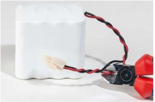
When purchased elsewhere, the 4S2P 14.8V/5.2Ah battery must be adapted to the connector of the IMAG-CM or IMAG-CG unit. To this end, remove the old battery as described on previous page. Individually cut the red and the black wire. Avoid short circuiting. Keep the disconnected plug.
