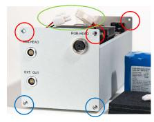
When ordered with WALZ, the battery is ready for installation. To change the battery, loosen the upper screws at front and back of the housing (red circles). Take off the housing cover. Disconnect battery! (See green circle.) Unscrew the screws at the bottom of the rear panel (blue circles).
