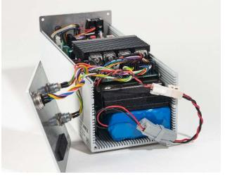
Strip end of wires. Use wire connectors to connect wires of the new battery to the wires of the old battery's plug. Connect wires of the same color. Make sure that the wires are firmly connected. Loose wire ends can get in contact with the housing or electrical circuits and entail serious damage.
