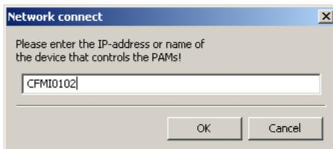
Generally, also the IP address can be entered in the Network connect window but only the DHCP host name provides a permanent address when different IP addresses are assigned to the MONI-IB4/LAN by the DHCP server.
