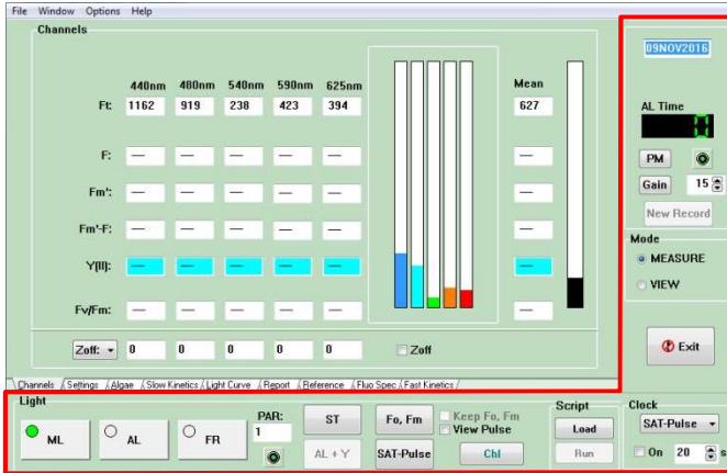
Fig. 11 User surface of PhytoWin_3 elements for system operation and display of instrument status
