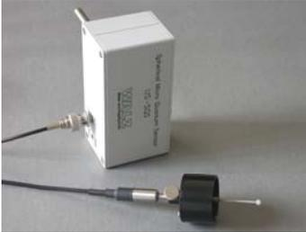
The US-SQS/B has a hood and an amplifier box, which contains a battery.
