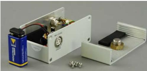
For exchanging the battery, unscrew all four screws at the top of the amplifier-housing. Take out the battery. Exchange it and put everything
