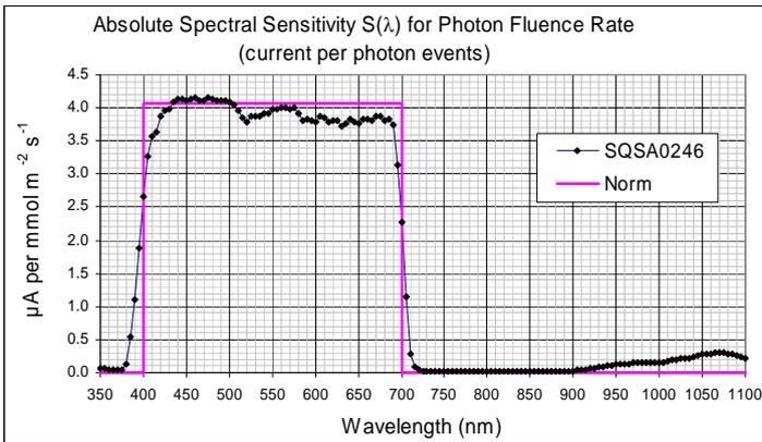
**Fig. 1a:** Absolute spectral sensitivity for Photon Fluence Rate
