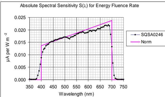
**Fig. 1b:** Absolute spectral sensitivity for Energy Fluence Rate
