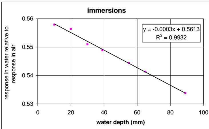
**Fig. 3:** Determination of immersion factor
