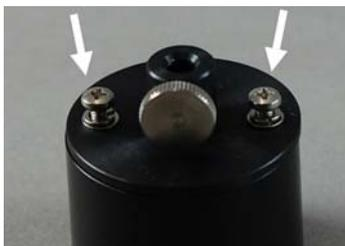
To remove the inner ring, unscrew the indicated screws. Afterwards use the screws to fix the upper plate to the threaded holes of the hood.
