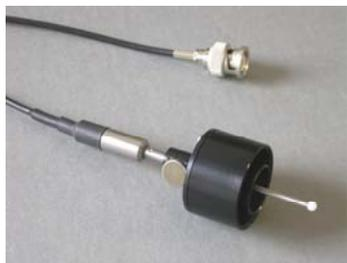
The US-SQS/IB has an adjustable black hood. The ULM-500 or another external data logger is required. The US-SQS/IB is recommended for the use with a PAM-100 or XE-PAM.
