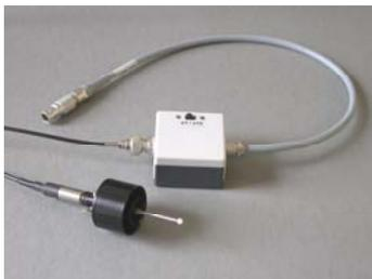
The US-SQS/WB has a hood and an amplifier box. With this amplifier box the light sensor can be connected to several PAM instruments. Technically the connection for the US-SQS/WB is the same as for the leaf-clip holder 2030-B. In particular the
