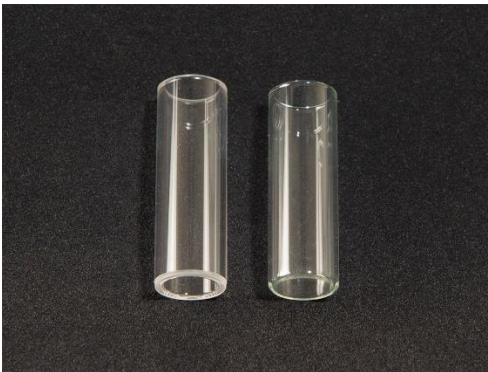
Fig. 2: stepped quartz glass bottom (left), continuous standard glass bottom (right)
