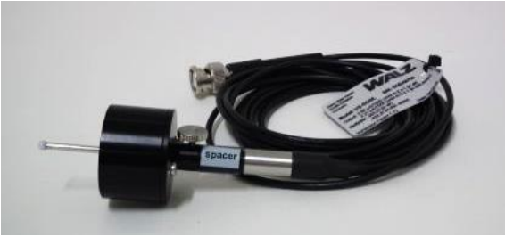
Fig. 3: US-SQS/L with spacer mounted between hood and sensor filter housing
